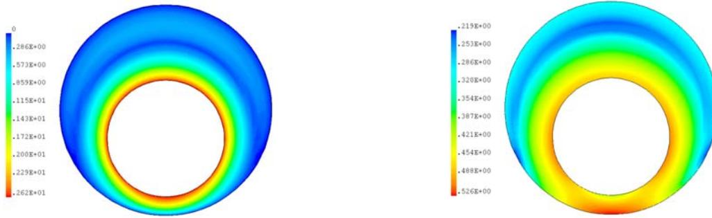
(b) Dilatant fluid, (left) Velocity field, (right) Viscosity field
