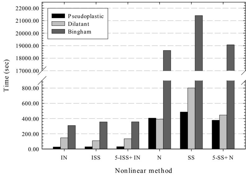
Fig.4 Nonlinear algorithms performance – CPU time (seconds) by method.
