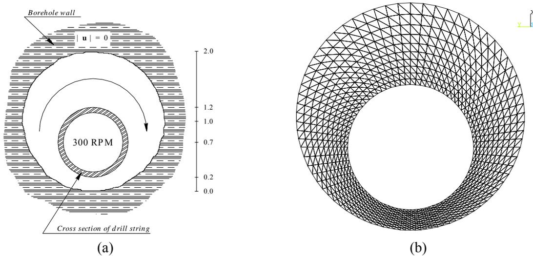
Fig. 1 (a) 2D cross section scheme of a borehole well showing the drill string at center and rotation direction. (b) Finite element mesh: 1,600 elements and 800 nodes.
